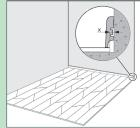
Before starting carefully measure the length and the width of the room to plan a precise lay-out to achieve a balanced appearance of the floor. This will ensure also you won't end up with the last row being too narrow. If the last row would be less than 100 mm the installation will be easier if you cut down the planks of the first row in the length.
