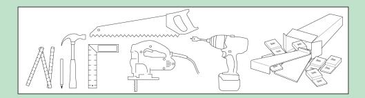
When cutting the Pergo wood plank be sure you are not creating splinters or chipping when cutting. If using a handsaw keep the decorative surface faced up. If using a jigsaw keep decorative surface down (except for a jigsaw with down-stroke blades).
