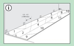
We recommend to install the first 3 rows first without using any adhesive. Please follow the sequence shown in the above picture. During installation, draw on the floor a line to mark where every panel ends. Once installed these 3 rows, uninstall the first row (panel 1 - 7) and the second row (panel 2-8) panel by panel. Row 3 needs to be kept in place. The result of these steps is a "drawn" Sandhamn floor on the subfloor. This will make the gluing process more efficient.
