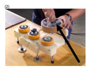
Now, the bending tool can be tightened again, repeat the action (1). The first and last 10 cm of the profile cannot be bent.
